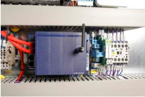
*More and more MICAFLUID machines are equipped with eWON Flexy routers, enabling them to communicate with IT systems and mobile devices over secure virtual private networks anywhere and anytime.*
