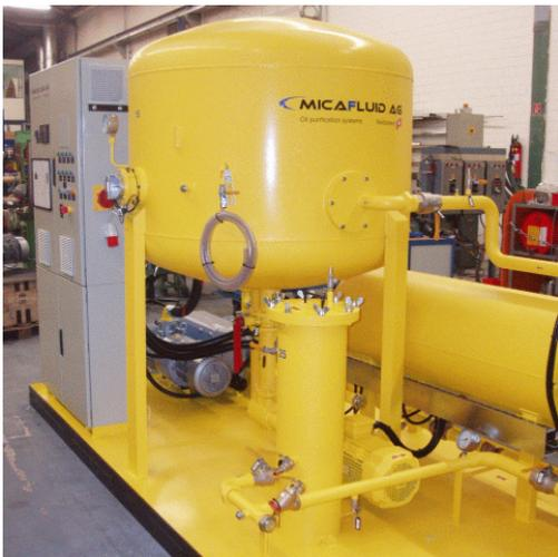
*The VOP oil treatment plant, which can be remotely controlled and maintained via eWON Flexy.*
